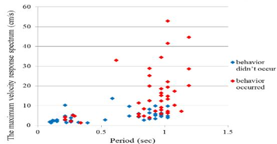
Figure 11: The relation between occurrence of abnormal behavior of water pressure and seismic characteristics of horizontal direction
