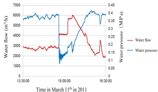
Figure 1 The transition of water flow and water pressure at Seibu water distribution station at the 2011 Great East Japan Earthquake
