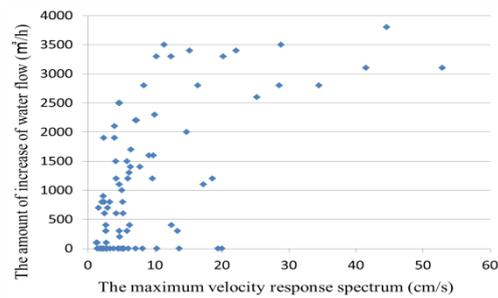
Figure 4: The relation between increase of water flow and the maximum velocity response spectrum of horizontal direction
