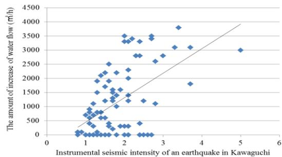
Figure 2: The relation between the amount of increase of water flow and the instrumental seismic intensity
