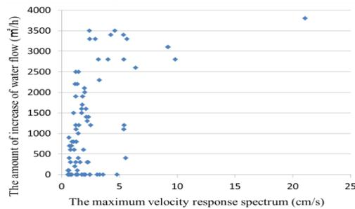
Figure 5: The relation between increase of water flow and the maximum velocity response spectrum of vertical direction
