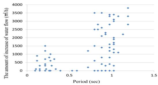
Figure 8: The relation between increase of water flow and the period of horizontal direction
