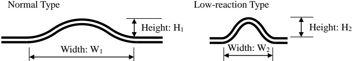
Figure 2 Reformed shape of Wave-shaped Pipe Section
