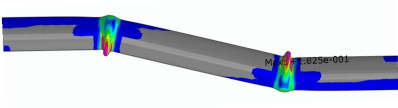
Figure 11 Result of FE Analysis in case of Spilt-basin Test
