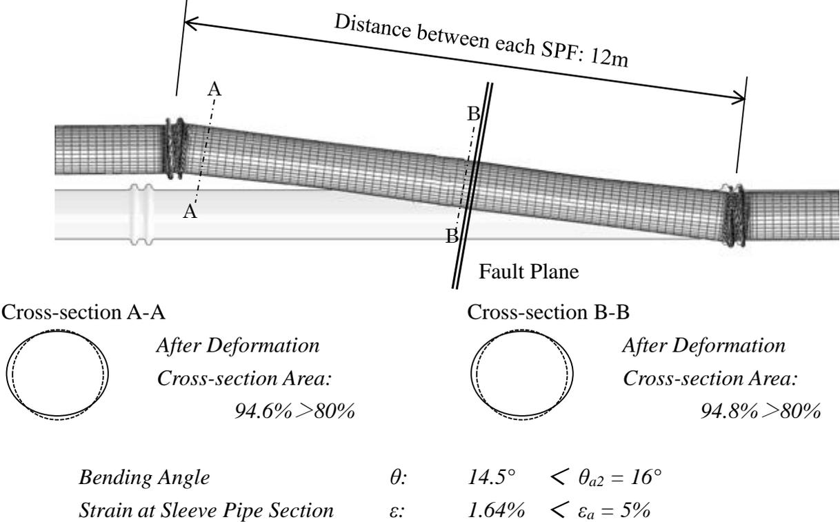
Figure 14 Cross-section area before and after fault offset
