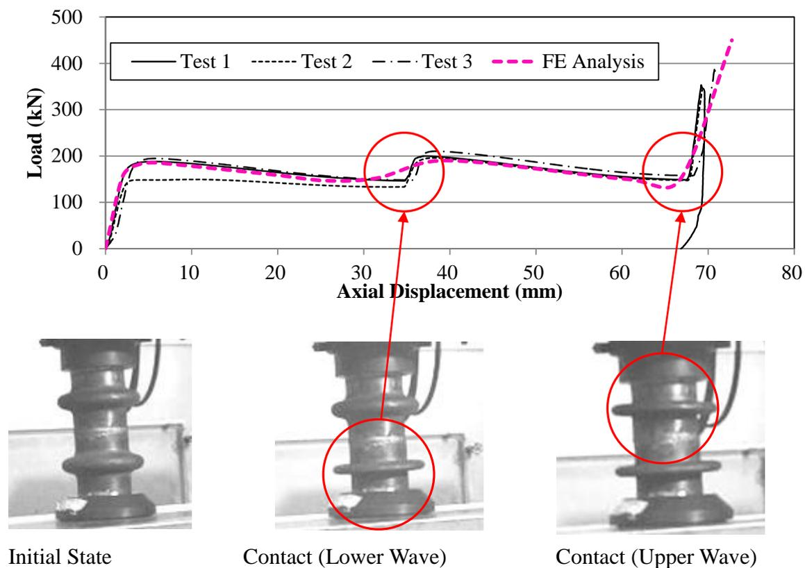
Figure 6 Results of Axial Compression Test
