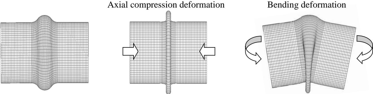
Figure 3 Deformation of Low-reaction Type of SPF
