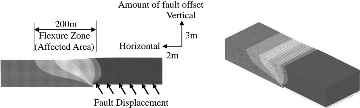
Figure 11 Distribution of Fault Displacement (Ground Deformation Analysis)
