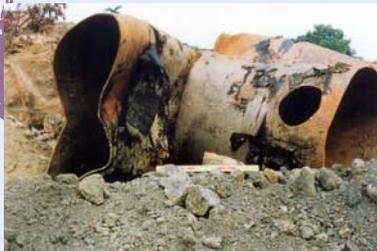
Damage to buried pipe by fault rupture
